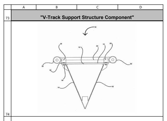
A track structure component having a triangular girder having a top plate, a first side plate and a second side plate, wherein a lower surface of the top plate abuts the first edge of the first side plate, the lower surface of the top plate abuts the first edge of the second site plate and the second side edge of the first side plate abuts the second site edge of the second side plate and a rail component having at lease one rail positionsed adjacent an upper surface of the top plate.
