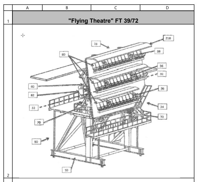
A motion base, comprising a pivot structure having a pivto point near the centre of gravity of the pivot structures, the platform having a generally horizaont position and a generally vertical position; and, a drive for rotating of the pivot structure at the pivot point to move the platform from the generally horizontal position to the generally vertical position.
